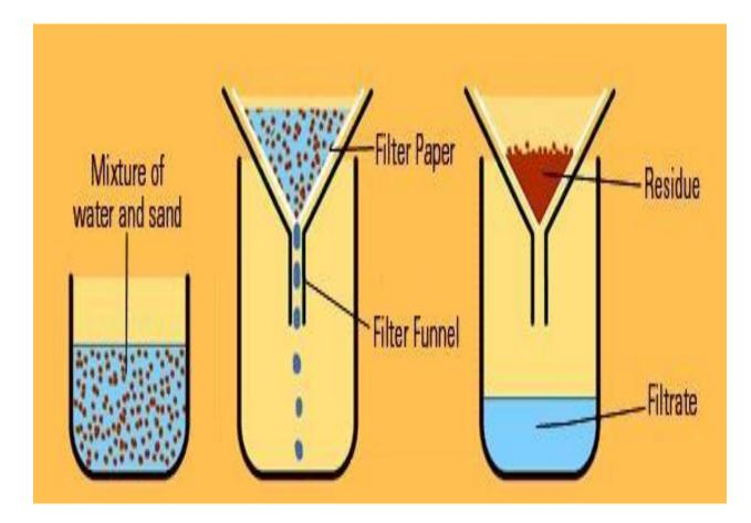
This process involves the use of a filter paper placed in a filter funnel. The funnel is placed in a beaker and the mixture of water and sand is poured into the funnel. The liquid part drains through the filter paper into the beaker, leaving the solid sand particles trapped on the filter. In filtration, the liquid part collected is called the filtrate and the solid bit that remained on the filter paper is called the residue.
